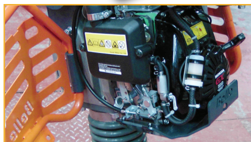
Dual Filtration Fuel System
