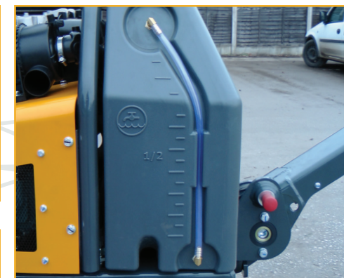
65 litre Water Tank with external gauge.
