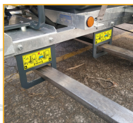
Forklift points for safe on-site transportation
