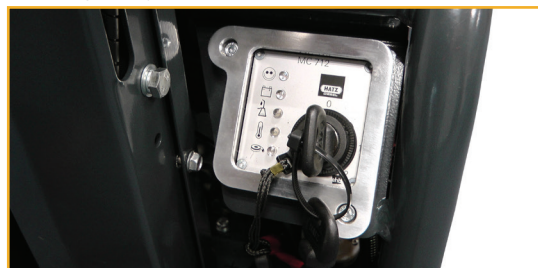
Electric, Key Ignition Start & Led Warning Lamps
