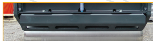
Self-Cleaning, Adjustable Scraper Bars
