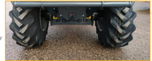
Wheel Spacer Option Adds 100mm To The Track Width Giving Added Safety & Stability
