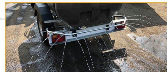
Gravity-fed spray bar option for dust suppression
