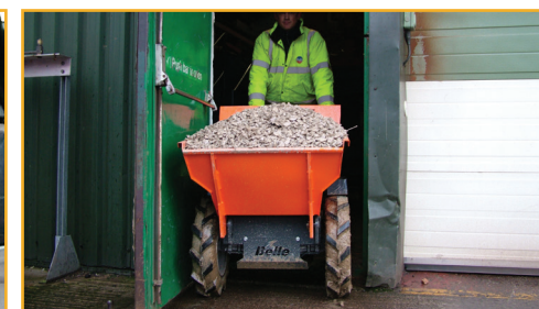
Designed to fit through a standard doorway
