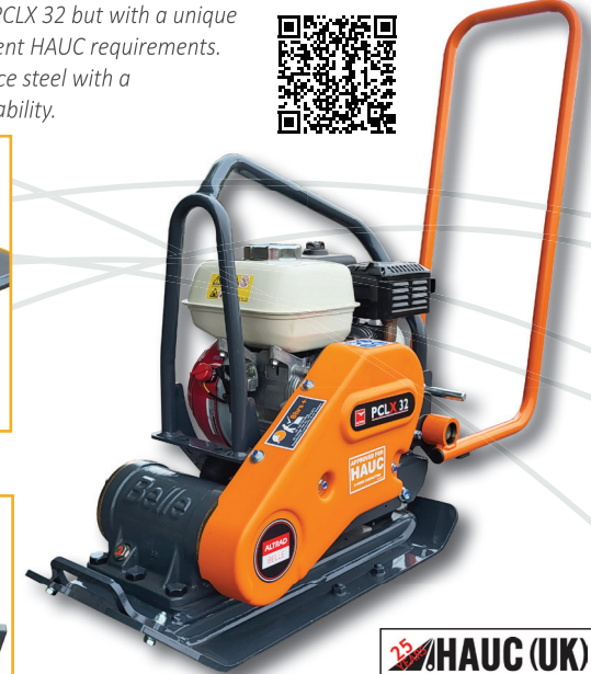
'Dual force' baseplate from Strenx™ performance steel with hardox® wear plate
