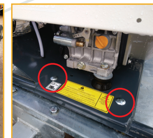
Anti-Theft Bolts Securing The Pressure Washer To The Chassis
