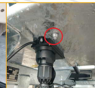
Anti-Theft Bolts Securing The Pressure Washer To The Chassis
