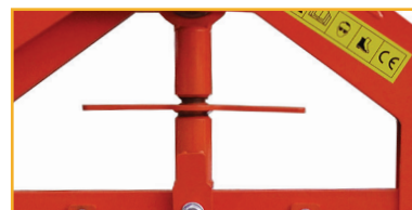
Large thread screw adjuster
