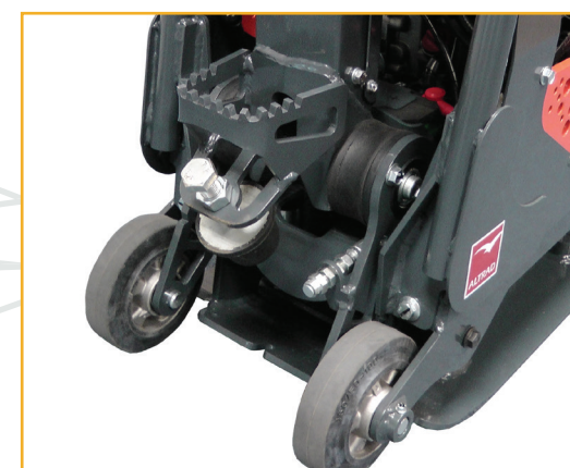
Integrated Wheel Kit & Foot Stand for Easy Transportation
