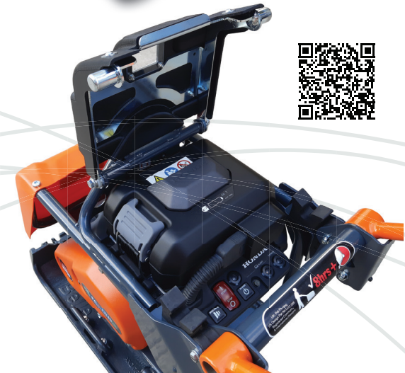
Battery power level indicator, always visible from operating position
