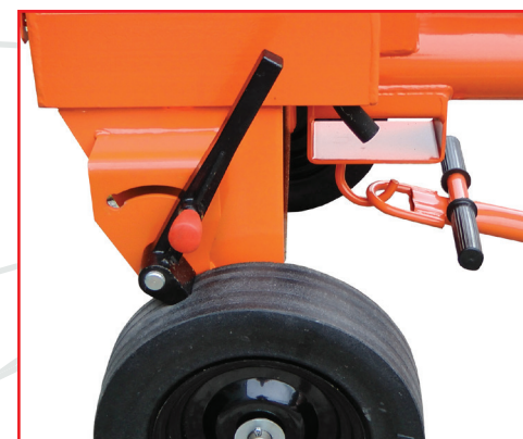
Parking brake for improved site safety
