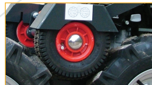
Carrier wheel disengages for easy wheel changing
