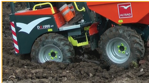
High-quality, all-terrain tyres with valve protect guard & wheel nut indicators
