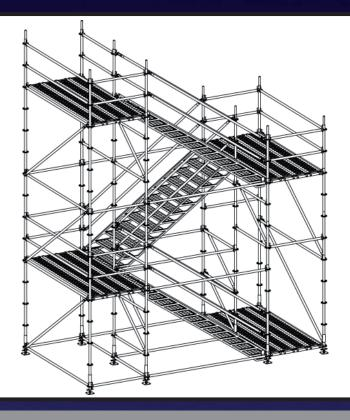
Load capacity 5.0 kN/sqm with stair width of 125cm. Load capacity 7.5 kN/sqm with stair width of 100cm.
