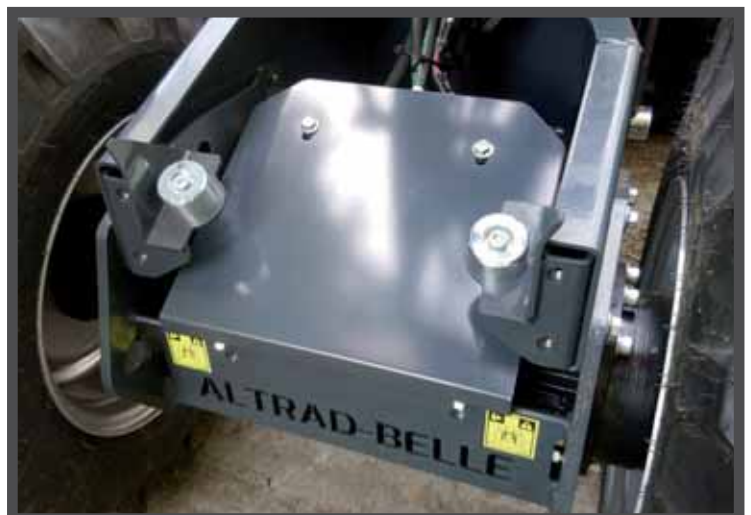
ROBUST STEEL, FRONT MATERIAL INGRESS GUARD PREVENTS DAMAGE TO HYDRAULIC CIRCUIT
