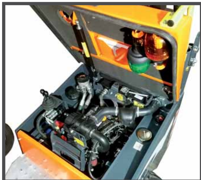
GOOD ACCESS TO KEY FEATURES WITH SELF-LOCKING GAS STRUT AND PROVEN YANMAR 3TNV76 DIESEL ENGINE
