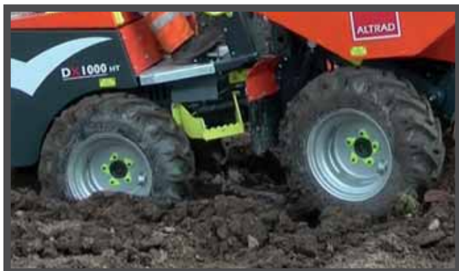
HIGH-QUALITY, ALL-TERRAIN TYRES WITH VALVE PROTECT GUARD & WHEEL NUT INDICATORS
