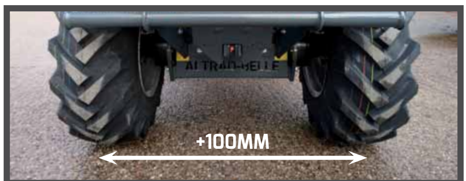
WHEEL SPACER OPTION ADDS 100MM TO THE TRACK WIDTH GIVING ADDED SAFETY & STABILITY
